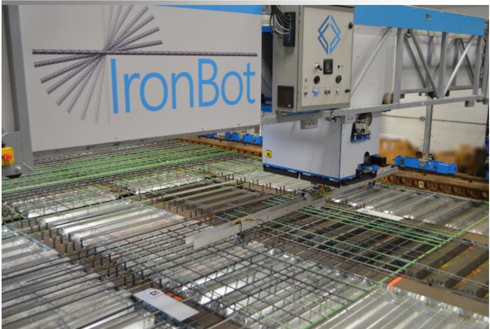
Rebar-placing robot unveiled at Bauma (GCR Staff, 2019)
